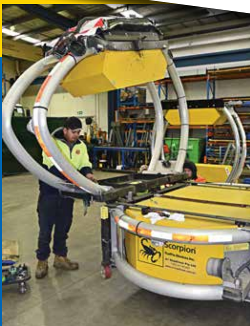
THE DAMAGED COMPONENTS BEING REMOVED FOLLOWING AN IMPACT.
