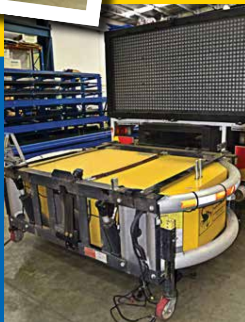
WITH THE DAMAGED COMPONENTS REMOVED, THE REMAINING SECTIONS ARE CHECKED PRIOR TO THE NEW COMPONENTS BEING FITTED.
